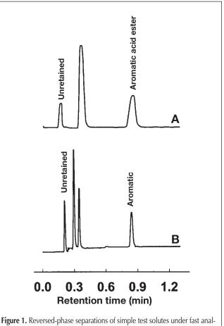
**Figure 1.** Reversed-phase separations of simple test solutes under fast analysis conditions. Chromatograms: (A)  $50- \times 4.6$ -mm i.d. column packed with 10-µm irregular octadecyl packing and (B)  $100- \times 4.6$ -mm i.d. RP-18 monolith column.
